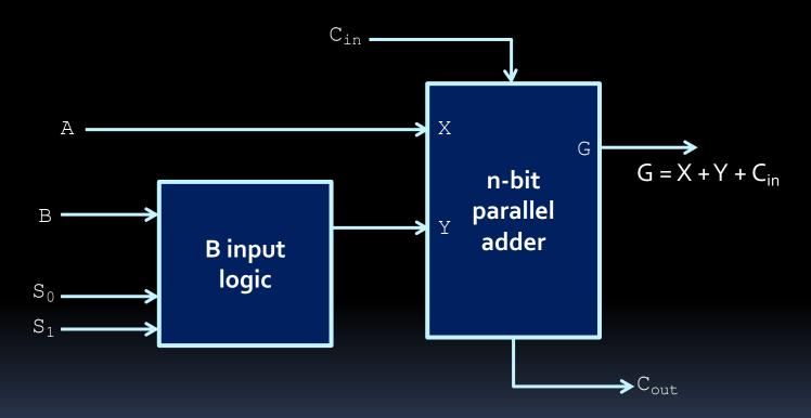
What values for S<sub>0</sub>, S<sub>1</sub> and C<sub>in</sub> do we need in order to subtract B from A?
