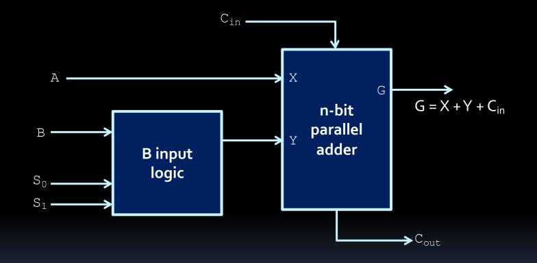
To subtract B from A, you must set S<sub>0</sub>=0, S<sub>1</sub>=1 and C<sub>in</sub>=1.
