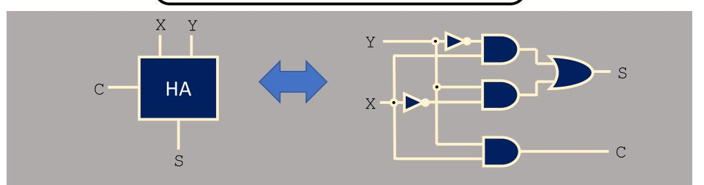
A half adder outputs a carry-bit, but does not take a carry-bit as input.
