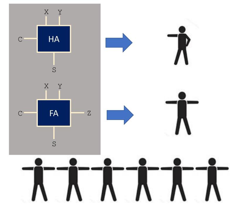
Each full adder takes in a carry bit and outputs a carry bit.
