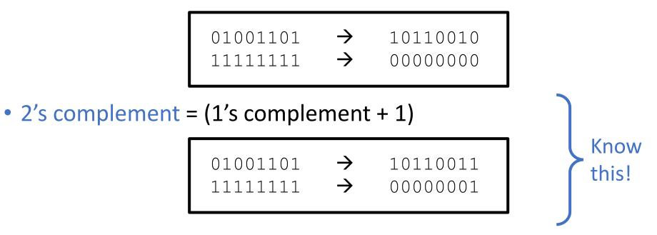
• <u>Note:</u> Adding a 2's complement number to the original number produces a result of zero.
