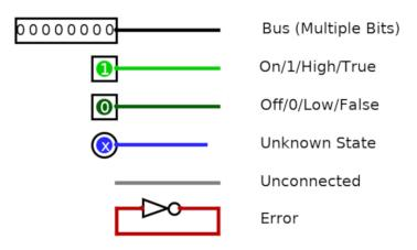
Wires and buses can have many states. You can inspect the state of a wire/bus using the  $\clubsuit$  "poke" tool available in the toolbar.
